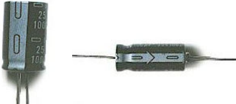
Tubular shaped For high voltage purpose Electrolytic capacitors
